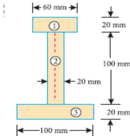
Q. 7 Find the centroid of the T-section shown in the figure below. All dimensions are given in the figure.
